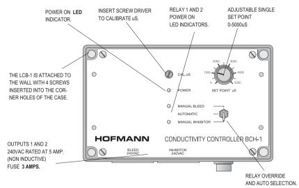
FIG. 2 FRONT PANEL LAYOUT
